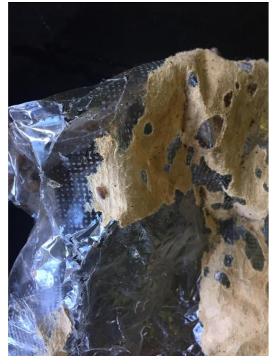
Here is a plastic purported to be plant-based and compostable, from a reputable health food company, clearly demonstrating after many weeks in a backyard compost system, that it is not truly biodegradable.
